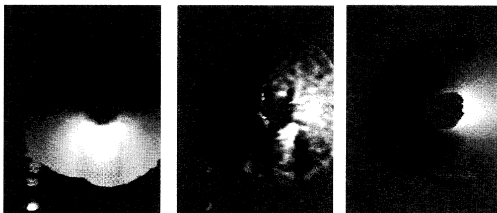
Fig. 6. Displacements measured in thick-walled tube phantom for frame corresponding to maximum compression. a) Interframe axial displacement, where white represents a downward displacement of 87.5 \mu\text{m} and black represents an upward displacement of 87.5 \mu\text{m} ; b) lateral displacement, where white represents a rightward displacement of 87.5 \mu\text{m} and black represents a leftward displacement of 87.5 \mu\text{m} ; and c) lateral displacement resulting from incompressibility processing of panel (b) based on the axial displacement of panel (a) using the same gray scale as panel (b).
