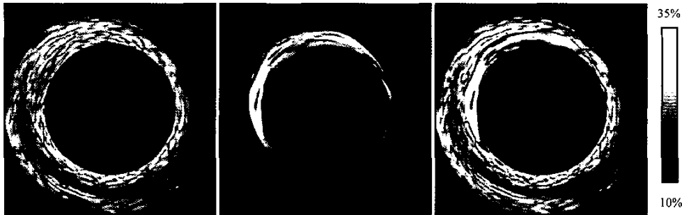
Fig. 10. Thrombosis in excised rabbit thoracic aorta. Left panel contains a B scan displayed over 40 dB. Middle panel contains a grayscale strain image displayed over a range of 0–35%. The right panel contains the B scan from the left panel superimposed by the strain image displayed in color (red scale) over a strain range of 10–35%. Dimensions of each panel are 8 mm \times 8 mm.
